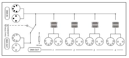
The physical signals of DMX512 are transmitted using shielded twisted pair wire. The controller and all receiving equipment are connected using "Daisy Chain" connections. The signal is jumped from the controller to a piece of DMX equipment then jumped to the next piece of equipment and so on. No branching is allowed. The final piece of equipment
