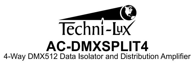
The AC-DMXSPLIT4 has One Input Port, 4 Optically Isolated Output Ports and user selectable Pass-Thru or Data-Termination. Except between the Input Port and Pass-Thru, each Port is electrically and optically isolated from the other Ports. All Ports have 3-pin and 5-pin connections, they are not isolated from each other and either the 3-pin or the 5-pin
