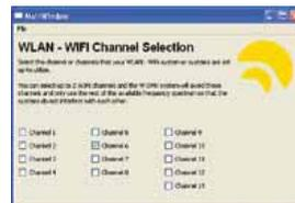
selecting which Wi-Fi channels are in use, and in the advanced mode, power users can disable individual W-DMX™ channels for finer control of the radio spectrum.
