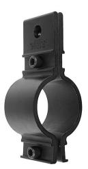
The two-piece, Mega Batten Clamp is great way to hang 1-1/2" pipe. The tight compression fit keeps pipe from rotating within the clamp. The Mega Batten Clamp wraps around the pipe batten on both sides and fastens with two 5/16"-18 TPI Socket Cap Screws using a 1/4" hex driver. Secure to structural supports through nominal 1/2" hole at top of clamp with up to a 7/16" shackle pin, quick link, or turnbuckle jaw. CNC Machined 3/16" thick x 2" wide 6061T-6 Aluminum.
