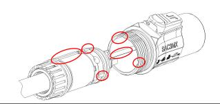
(5) After the assembly of the strain relief, inner core component and housing, tighten the boot in a clockwise direction with a torque of 2.0 Nm.
