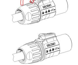
Note: This product is equipped with two sizes of waterproof rubber rings on the strain relief as standard. They are applicable to different cable diameters and can be replaced by the customers according to the diameter of the cable used, as shown in the picture.
