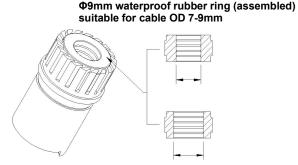
Φ11mm waterproof rubber ring (accessory) suitable for cable OD 9-11mm
