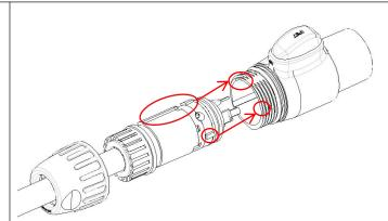
(5) After the assembly of the strain relief, inner core component and housing, tighten the boot in a clockwise direction with a torque of 2.0 Nm.
