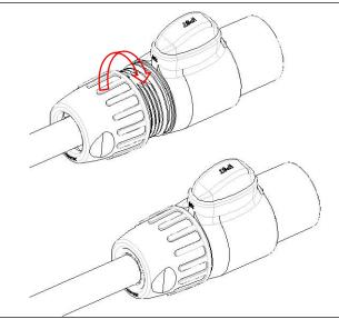
Note: This product is equipped with two sizes of waterproof rubber rings on the strain relief as standard. They are applicable to different cable diameters and can be replaced by the customers according to the diameter of the cable used, as shown in the picture.
