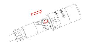
(6) After the assembly of the cable clamp, inner core and housing, tighten the boot in a clockwise direction.
