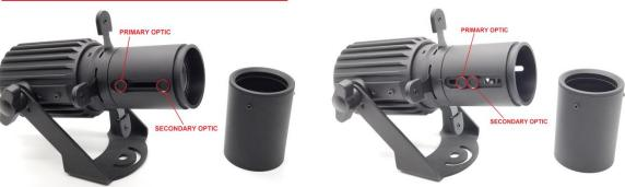
To widen the beam move the primary optic forward about 1 mm, and then move the secondary object backward along the optic slider rails toward the LED until the beam comes back into focus. Repeat this process until you have your desired projection size. At the maximum beam size, the primary and secondary optics will be touching each other at about  $1/3_{rd}$  of the length of the optic slider rails.
