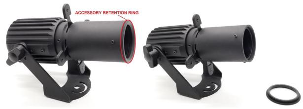
Once the retaining ring is removed, the accessory can be inserted. Place the accessory in the desired orientation, then tighten down the retaining ring.
