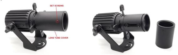
Power on the fixture. Be sure to never look directly at the LED while the fixture is on. Now, move the primary optic as close to the LED as possible and the secondary optic as far from the LED as possible on the optic slider rails. Slowly begin sliding the secondary optic toward the LED until the projected image comes into focus. This will be the narrowest focused beam the fixture can achieve.
