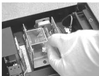
Installing the Lamp (EHJ)
